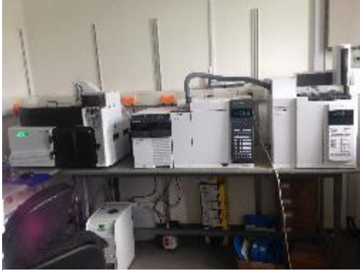
L- R High performance liquid chromatography; Liquid Chromatography Mass Spectrometer; Gallery plus Spectrometer in Entebbe laboratory Wakiso district
