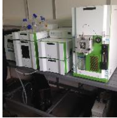
L- R High performance liquid chromatography; Liquid Chromatography Mass Spectrometer; Gallery plus Spectrometer in Entebbe laboratory Wakiso district
