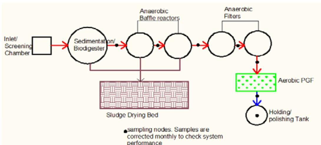
**Figure 40: Schematic layout of the DEFAST**
