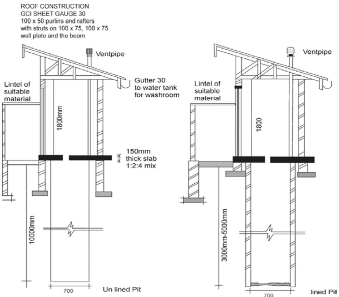
**Figure 28: Ventilated improved pit (VIP) latrine with unlined pit (left) and lined pit (right)**
