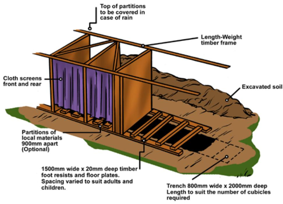
Figure 26: Typical design and layout of a trench latrine
