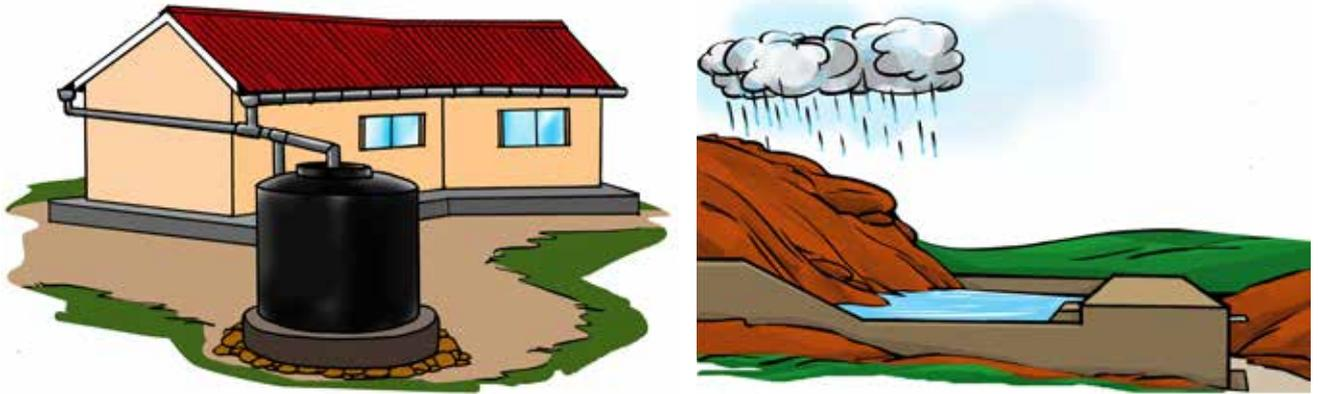
**Figure 2: Roof catchment (left) and rock catchment rainwater harvesting system**
