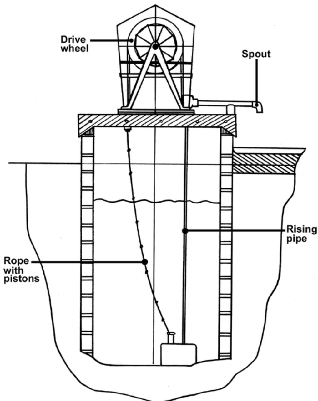
**Figure 18: Rope pump installed on a dug well**
