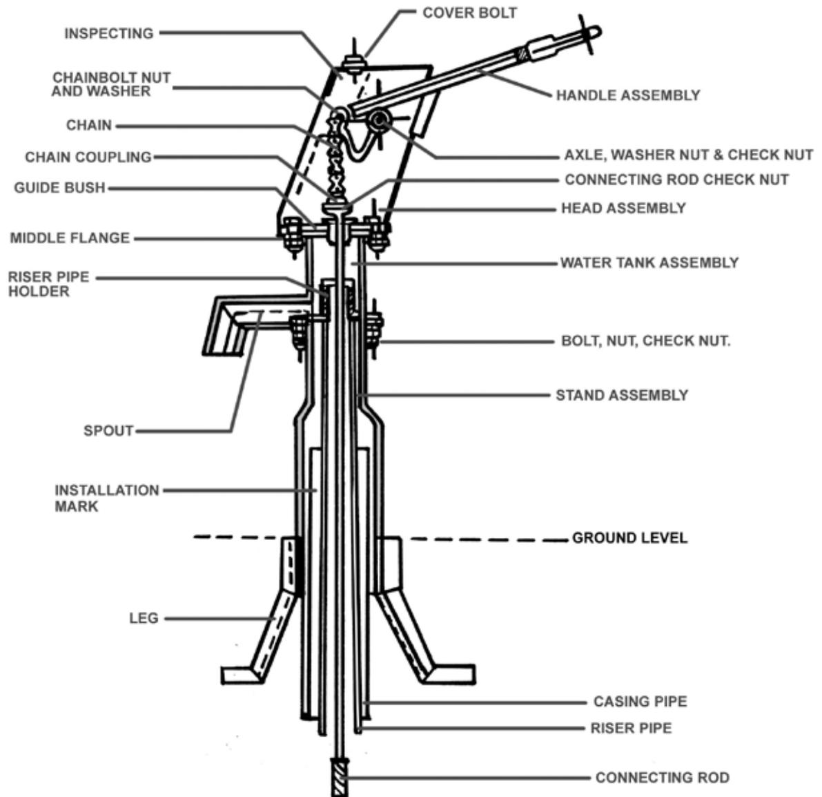
Figure 16: Pump head assembly
