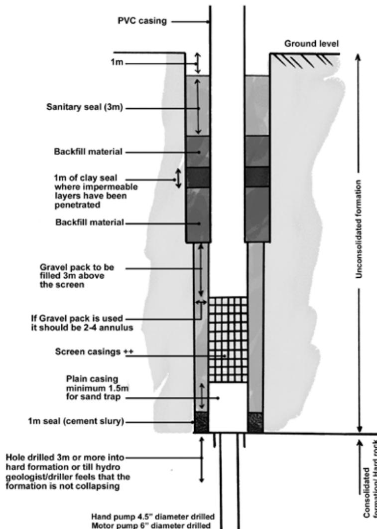
Figure 15: Detailed outline design and installation of borehole
