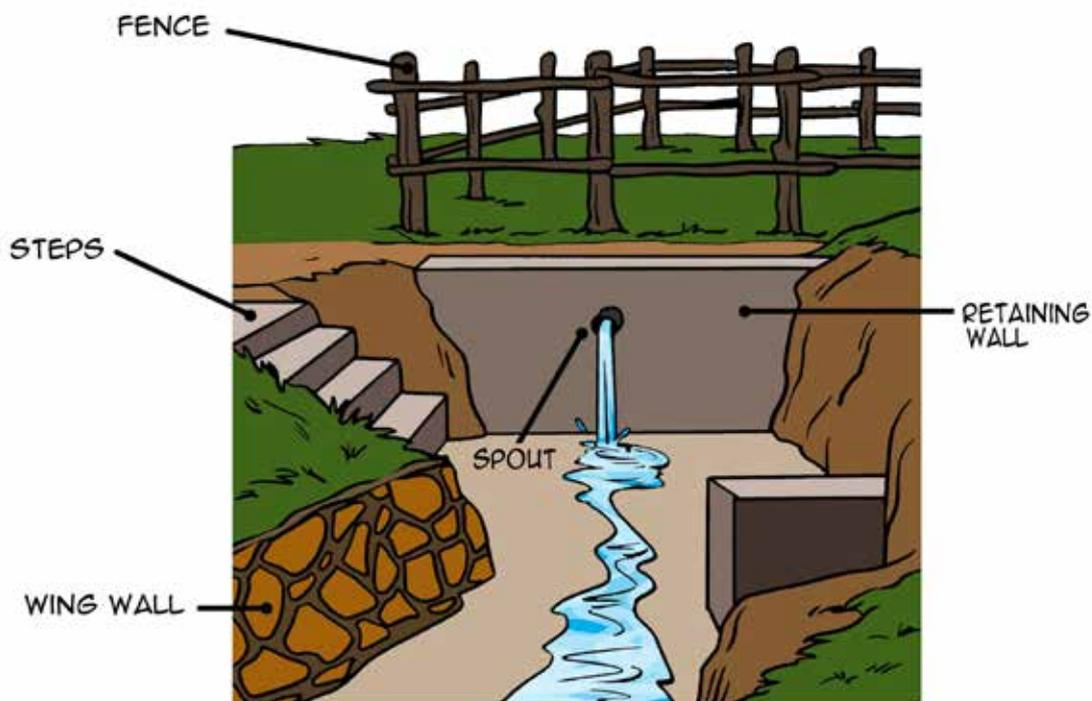
**Figure 11: Ordinary Spring construction (for high-yield springs)**
