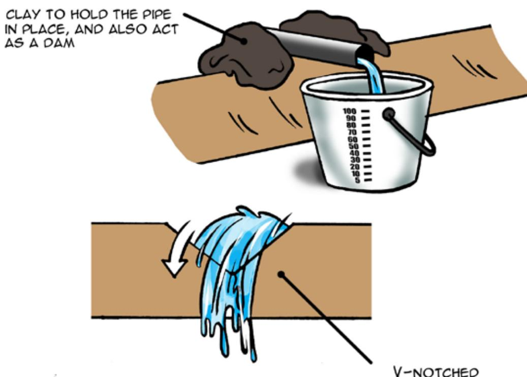
**Figure 10: Measuring yield of a spring well**
