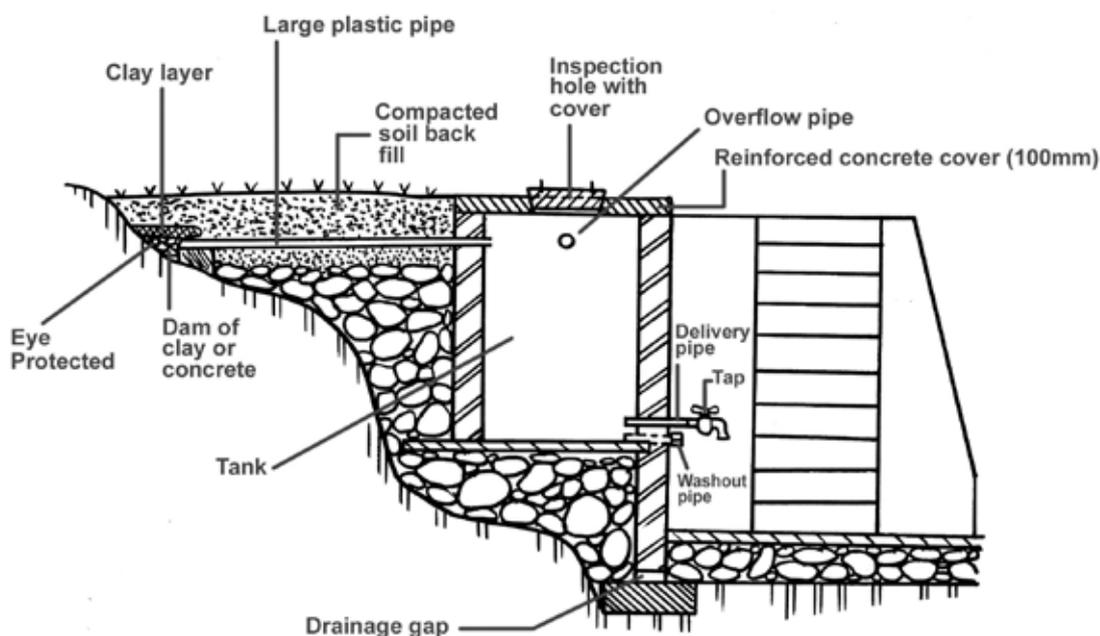
**Figure 12: Spring Tank construction (for low-yield springs)**
