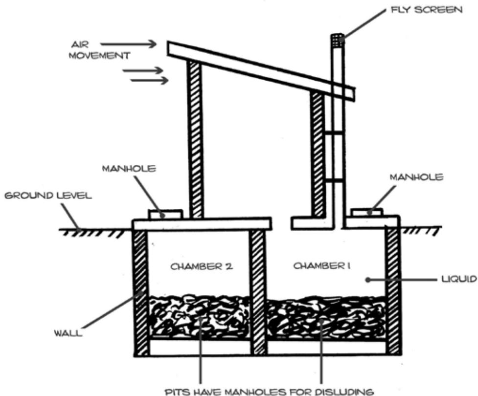
Figure 33: Alternating pit with two chambers
