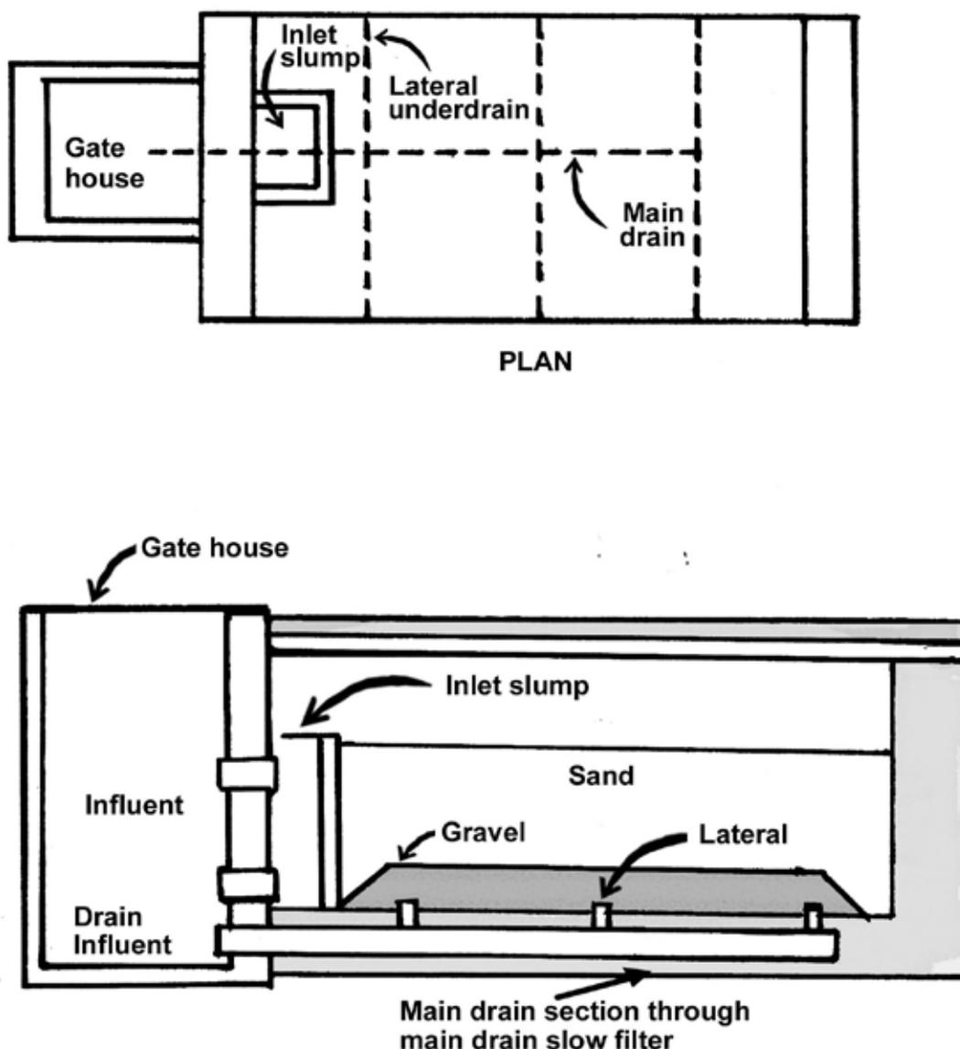
Figure 21: General layout and components of slow sand filter
