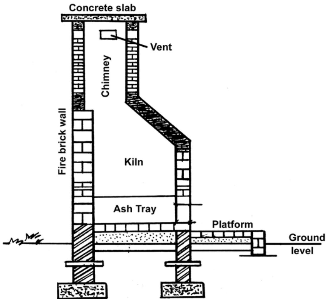
Figure 47: Typical single combustion chamber incinerator
