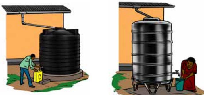
**Figure 5: Plastic tank (left) and stainless steel tank (right)**
