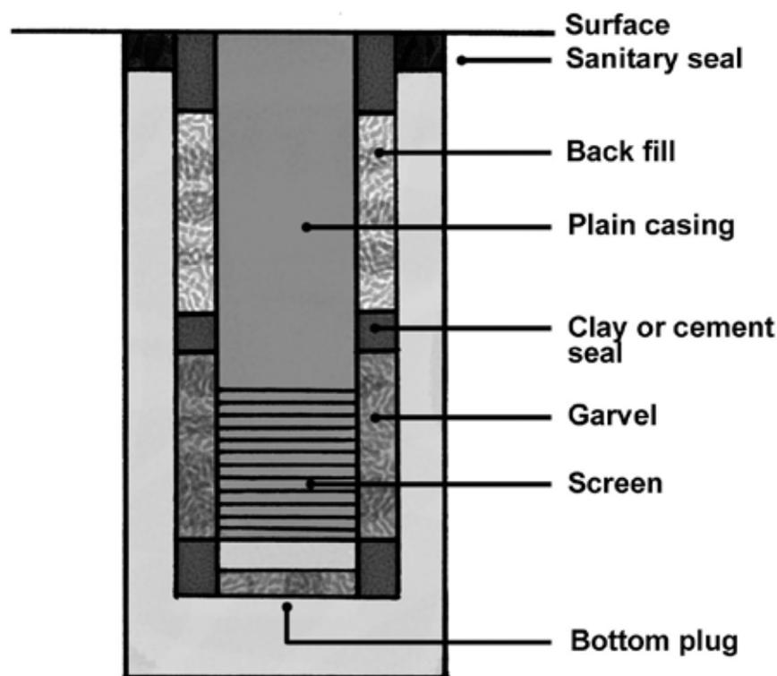
**Figure 14: Tube well design and installation**
