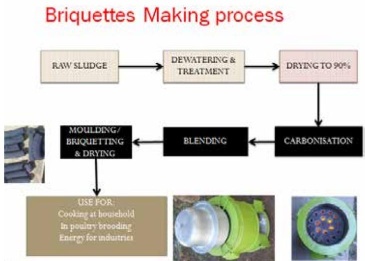
Figure 41: Processes of making faecal reuse products (Water For People Uganda, 2016).
