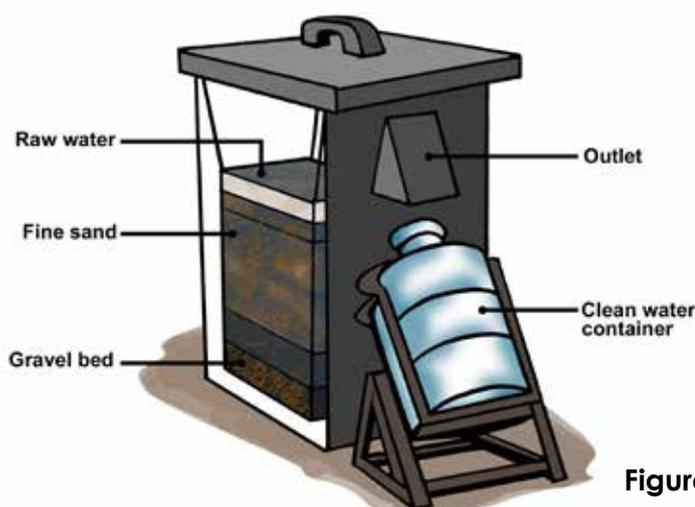
Figure 23: Bio-sand filter
