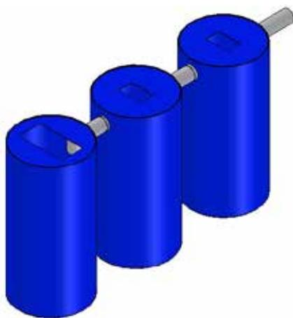
**Figure 37: Pour flush latrine with barrels as septic tanks**
