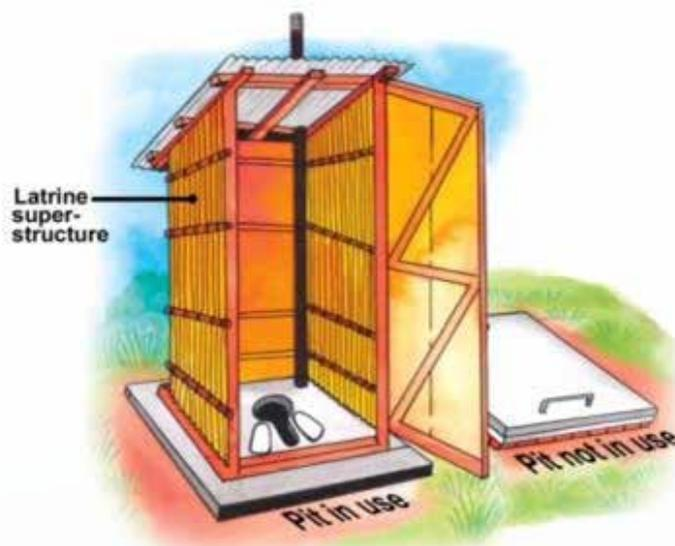
Figure 31: A typical layout of the Fossa Alterna toilet
