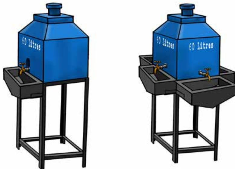
Figure 45: HWF with multiple taps (left) and with a single tap (right)
