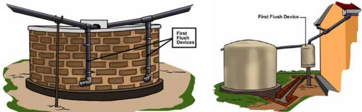
**Figure 7: Small capacity FFD (left) and large capacity FFD with washout valve**
