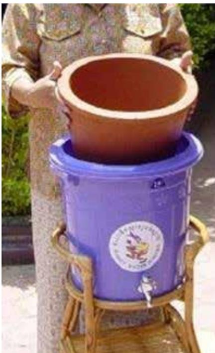
**Figure 24: Placing the ceramic vessel into the receptacle**
