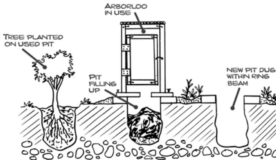
Figure 29: Schematic Diagram of an Arborloo
