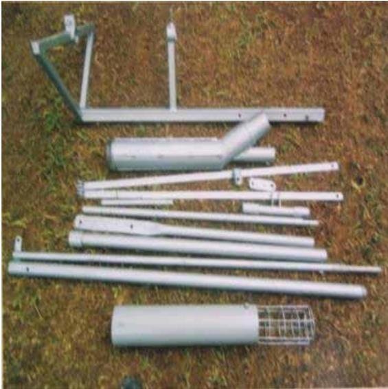
**Figure 39: Components of the Gulper II (as assembled above)**
