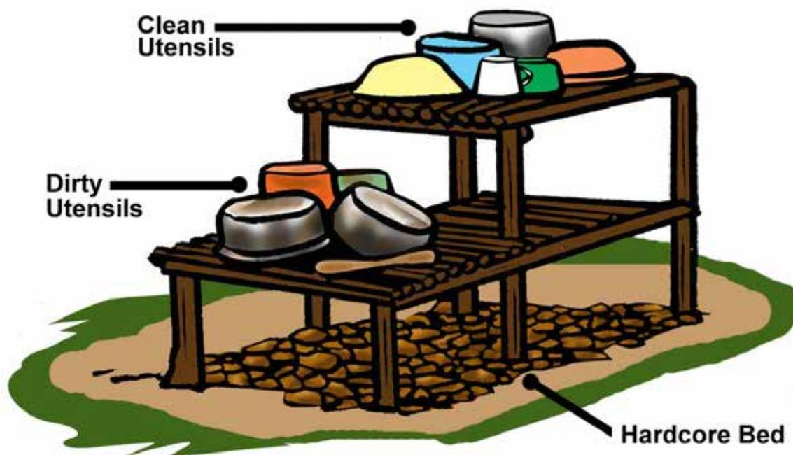
Figure 49: A typical drying rack
