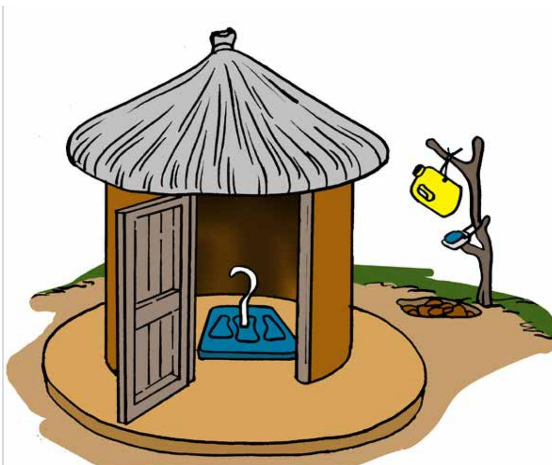
Figure 27: Typical traditional pit latrine improved with SanPlat
