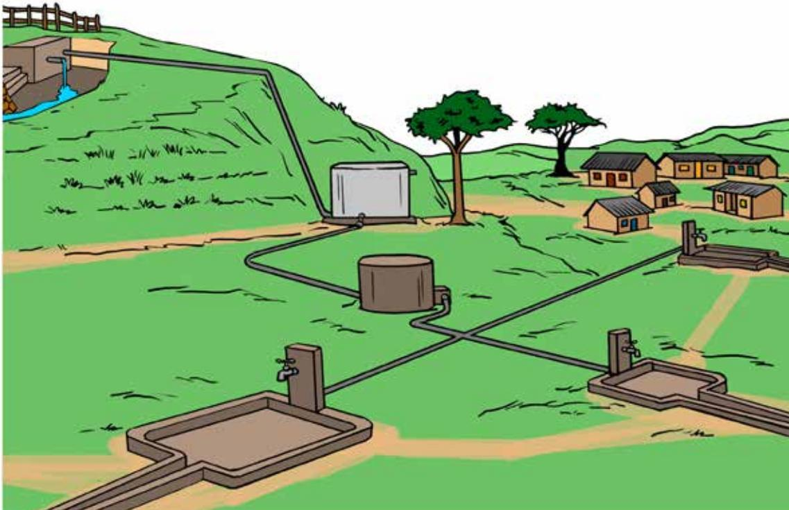
Figure 19: Schematic presentation a gravity flow scheme
