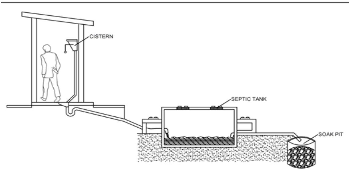
**Figure 34: Diagrammatic representation of a septic tank system**
