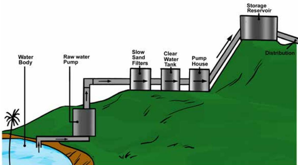
Figure 20: Diagrammatic representation of a piped water supply system
