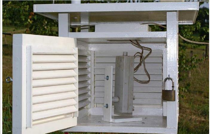
The floor should not be plain to further allow aeration and also to avoid damaging the devices in case water should nevertheless enter the shelter.
