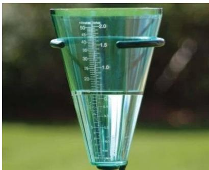
**Fig. 7-4: Rain gauge reading**
